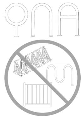
Figure 2. Recommended (top) and not recommended (bottom) bicycle rack designs. Source: DMMC
