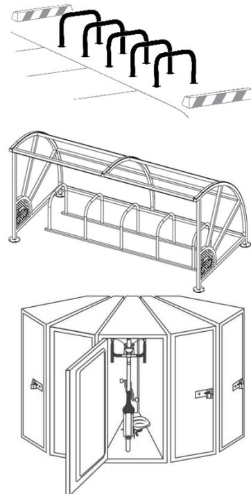
Figure 1. (top) corral of bicycle racks; (middle) sheltered bicycle rack; (bottom) bicycle storage locker. Sources: APBP, DMMC
